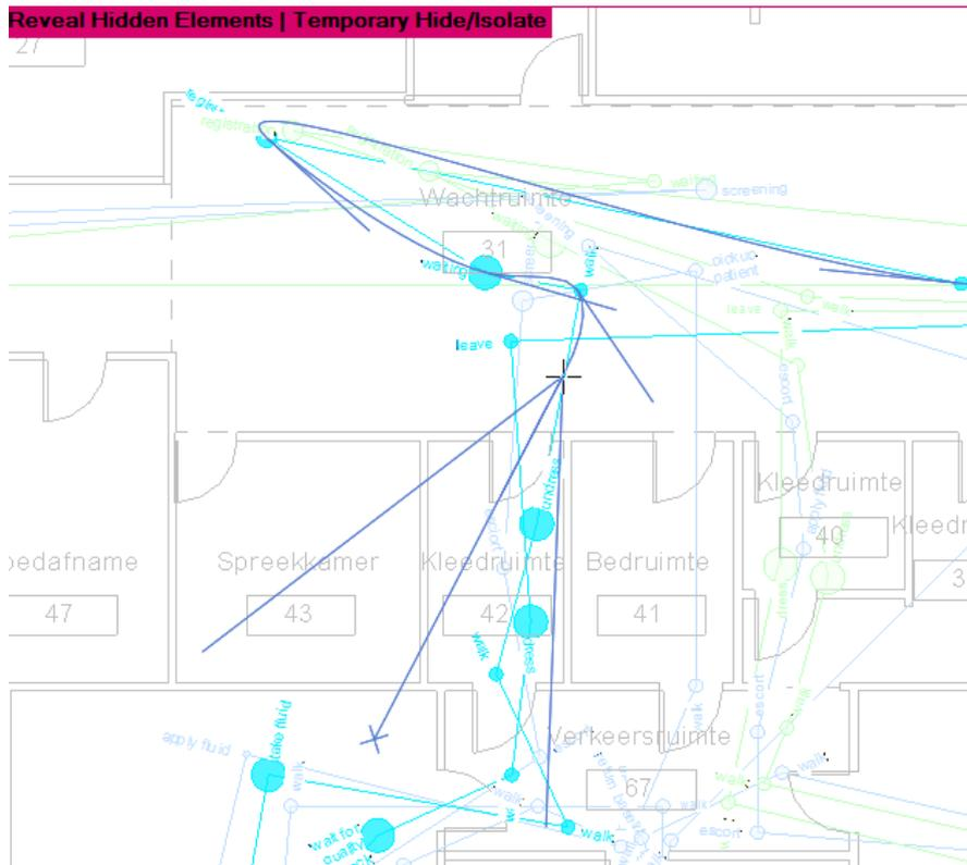
After you finished, you can test or adjust your walkthrough by clicking in **Edit Walkthrough**. Rewind to the **Previous Key Frame** and **Play**.
