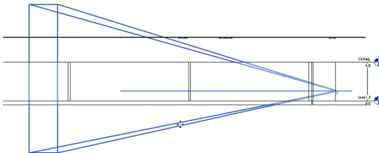
If you want to see only one path in the walkthrough, add filters at the Visibility/Graphic properties. Hiding doors is very important because Revit doesn't open them. The user can get very confused after crossing a closed door in a walkthrough. Avoid that by putting Doors 100% transparency at the Model Categories tab.
