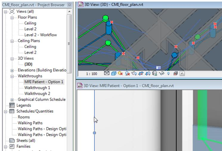
The standard height for the first person perspective might not be appropriate to give a good sense of spatial dimensions. You can lower the whole walkthrough by switching to an elevation view.
