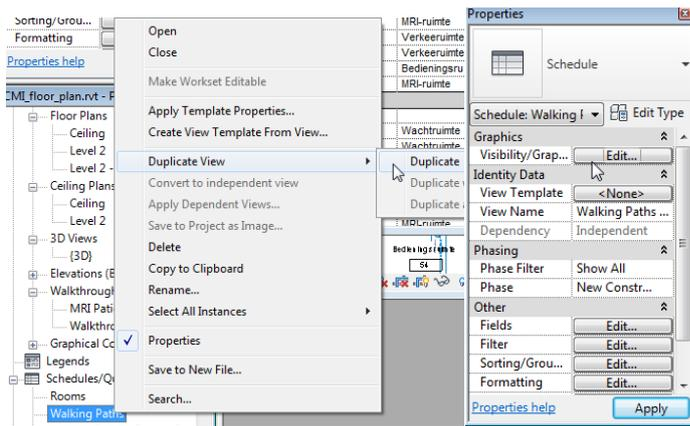
For each option, you need to create a new schedule. You can display a summary of the paths by unchecking the option **Itemize every instance** in Sorting/Grouping schedule properties. In that case, you should also remove the parameters **Step** and **Room:Name** from your schedule in Fields tab. As you can see from the example below, the second design option reduces nurse walking distance, but increases it for patients.
